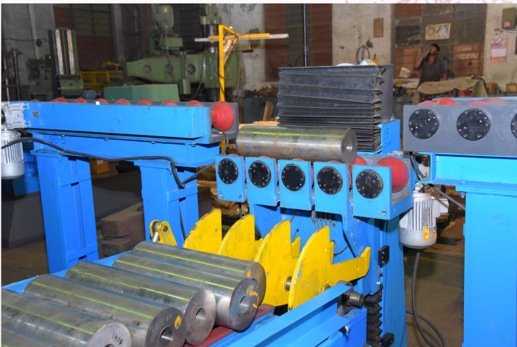
Billet Unloading Table with Additional Conveyors
